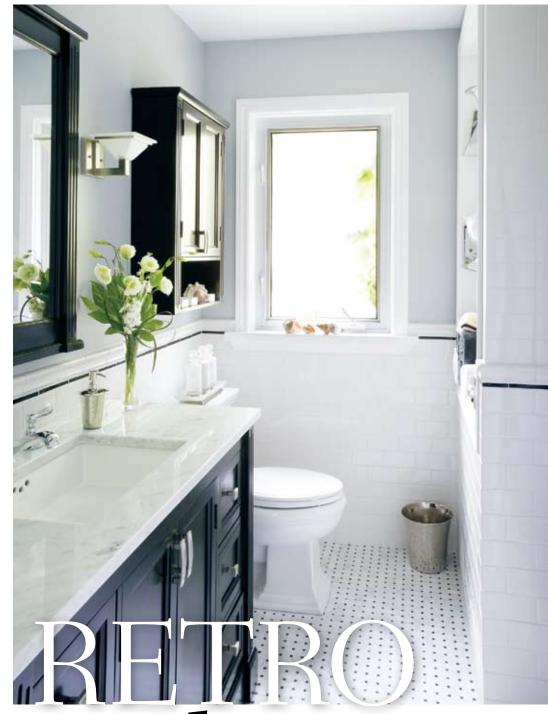
The eight- by five-foot footprint, plumbing locations and window are the only elements that weren't changed. Plaster walls were stripped to the studs and replaced with drywall, the wood floor was replaced with a new subfloor, and all fixtures were replaced. Wiring and plumbing were upgraded, and a new Broan exhaust fan, plus pot and accent lighting, were added.
